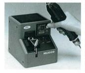
Set the Preset Knob to the number of screws you desire to be fed with, and turn on the Power Switch for the Counters. Press the Clear Button to set the reading of the Positive Counter to zero, then turn the Reset Button to adjust it to the same number that has been set on the one-digit Negative Counter.
